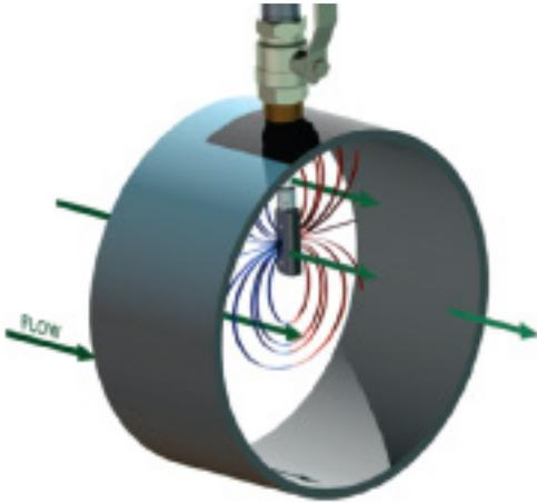
on plastic pipes, the electromagnetic flow meter requires electrical grounding by connection to grounding rings or ground probes inserted into the pipe. Readings are not affected by the fluid temperature, pressure, or viscosity.
