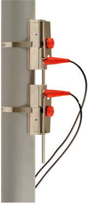
The choice of V, Z, or W mounting method depends on the application and pipe diameter. V-mount is the most common method while Z-mount is used for larger pipes or weak signal applications and W-mount for smaller pipes.
