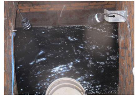
dBi-M3 MicroFlow-i area velocity monitoring
